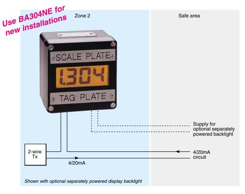
The BA304NC is a Type nL certified field mounting indicator which displays the current flowing in a 4/20mA process loop in engineering units. This indicator has a 25mm high 3½ digit liquid crystal display and is available in an IP66 aluminium or GRP enclosure.
